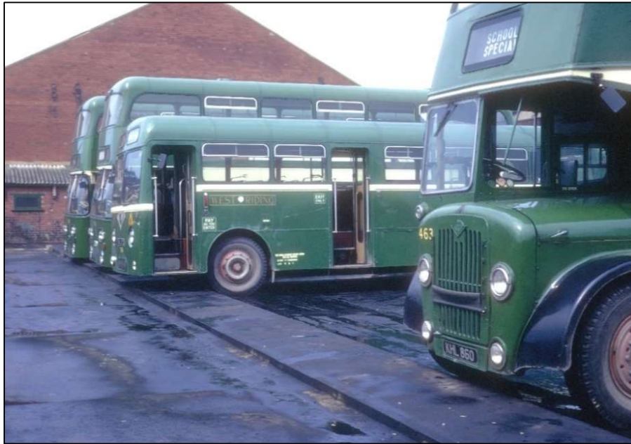
Two of the bus types mentioned above are seen at Featherstone depot on 13 June 1972. On the right is Guy Arab IV-Roe 463 (ex-860) and next to it is AEC Reliance 2MU3RV-Roe 104 (ex-923) sporting the last type of West Riding fleetname before NBC liveries took over. Beyond are Roe-bodied Daimler Fleetlines 635 (200) and 638 (203). What colour and pattern of moquette did the first two buses have when new? Despite the green livery being on the way out, all four buses are very well presented. (Basil Hancock)
