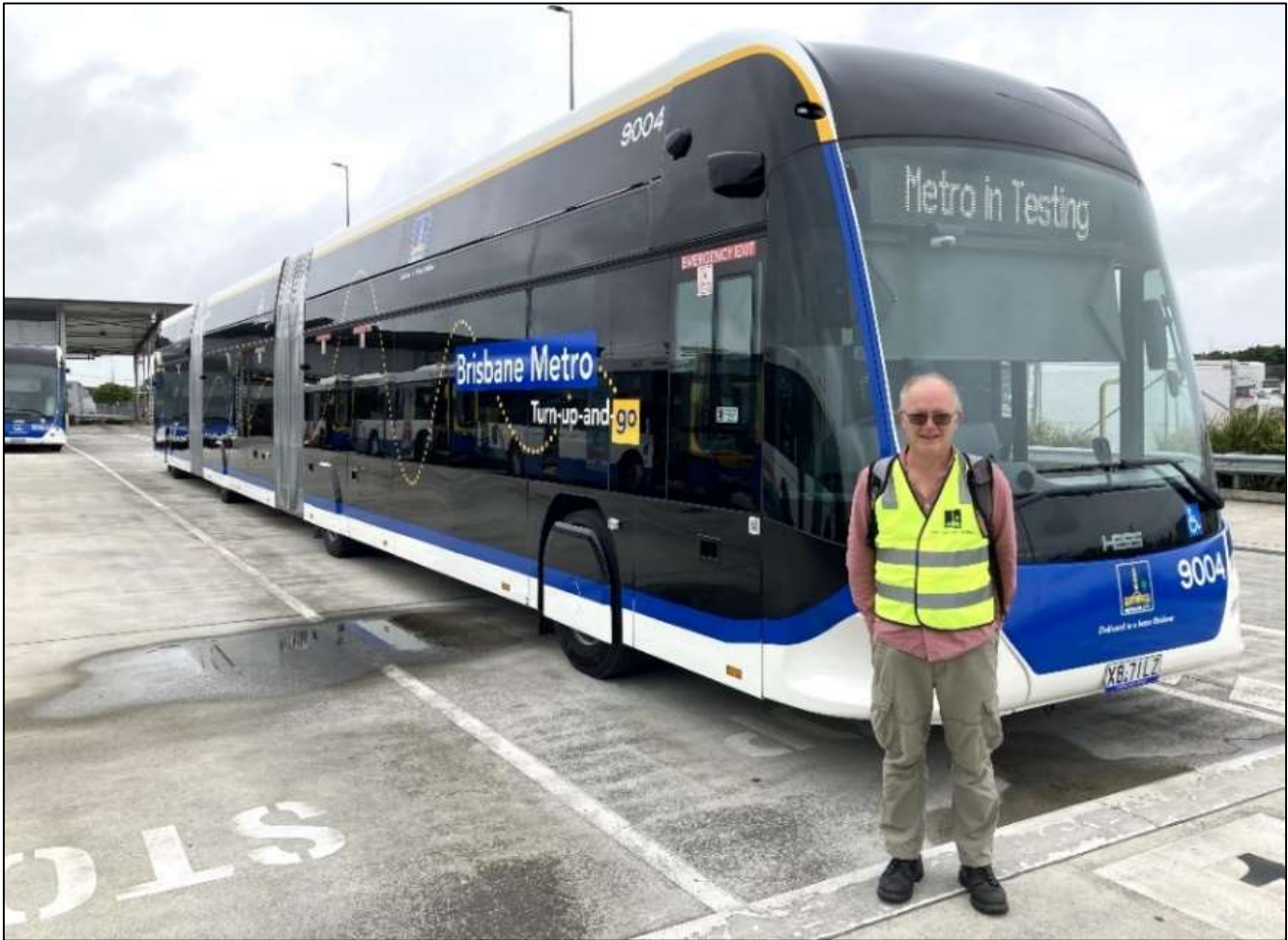
The editor in February 2024 standing in front of Brisbane Metro three-section articulated electric bus, 9004, one of 60 Hess Lightrams being delivered for the Metro busway network, which opens later this year. He spent three years working on the project as the lead vehicle technical engineer. It combines his current interests in zero emission buses and bus rapid transit. The Metro name of the operation replicates that of the former West Yorkshire PTE, but has been chosen to differentiate what will be effectively a rubber tyred light rail service from the usual buses that the City Council also operates, in some cases over the same busways. (Basil Hancock)
